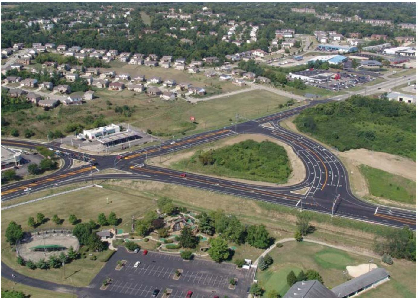
Figure 2: Aerial view of the completed quadrant roadway intersection (QRI) in Fairfield, Ohio
